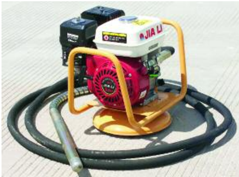
Figure 11.7 – Immersion type concrete vibrator with gasoline engine
